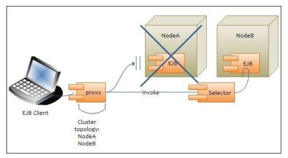
If a suitable node is found, the **JBoss EJB Client** implementation creates a connection to that node (in our case **NodeB**) and creates an EJB receiver out of it. At the end of this process, the invocation has now been effectively failed over to a different node within the cluster.
