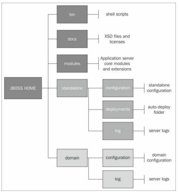
As you can see in the preceding diagram, the WildFly directory layout is divided into two main parts: the first one is pertinent to a standalone server mode and the other is dedicated to a domain server mode. Common to both server modes is the modules directory, which is the heart of the application server.
