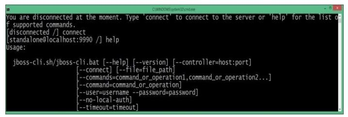
We started an interactive shell session that can also use the command-line completion (by pressing the *Tab* key) to match partly typed command names. No more searches are needed to find the exact syntax of commands!
