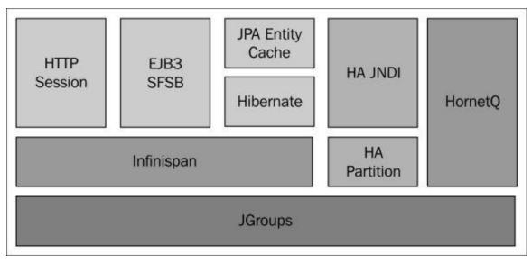
The backbone of JBoss clustering is the **JGroups** library, which provides communication between members of the cluster using a multicast transmission.
