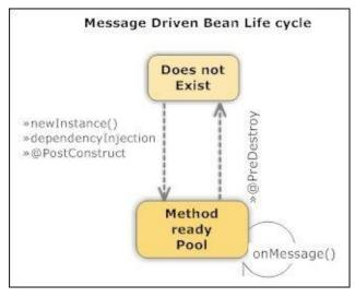
When a message is received, the EJB container checks to see whether any MDB instance is available in the pool. If a bean is available in the free pool, JBoss uses that instance. Once an MDB instance's onMessage() method is returned, the request is complete and the instance is placed back in the free pool. This results in the best response time, as the request is served without waiting for a new instance to be created.
