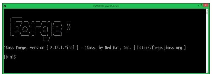
The console accepts a large set of commands, such as commands to navigate and manipulate the filesystems, to create new projects, to operate on the Forge environment and UI generation, and scaffolding commands. It also offers the autocomplete feature.
